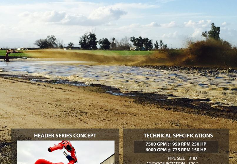
Conventional centrifugal pumps only have one discharge on the housing. That means that for every rotation of the fan, the pump is wasting power by trapping manure and not allowing it to easily get out of the housing. By adding multiple outlets, the manure is able to get out of the housing faster, resulting in pumping greater volumes with less horsepower.
