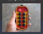
**RADIO CONTROL** Optional wireless control of valve to switch from "agitate" to "fill"
